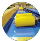
Driver-side guide rail covered with UHMW plastic to protect rims.
