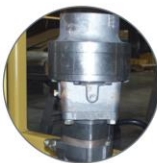
Heco direct drive gear box with hydraulic motor.
