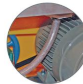
Pump is gravity-fed from tank.
