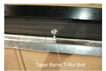
**Note:** The Taper Barrel nuts will need to be hammered into the bottom side of the UHMW cover.
