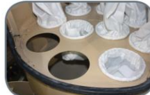
New and improved composite metal bag holder
