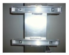
2. Insert the screws with the flat washer and lock washer into the Cyclone mounting brackets and hand tighten to the post unistrut nuts.
