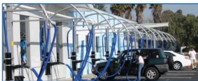
Vacuum booms with dual drops without canopies
