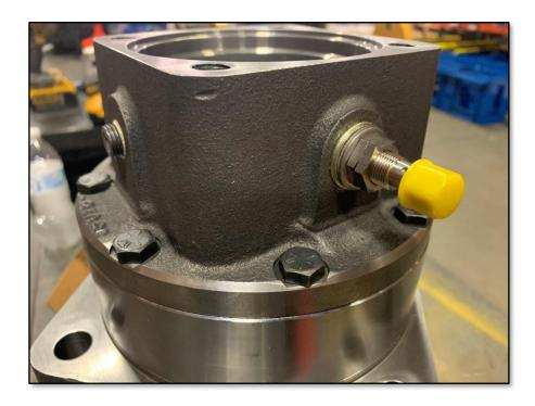
**Note**: The Pulse Speed Sensor should point towards one of the 4 attachment bolts on the HECO Gearbox and roughly 45 degrees away from the keyway of the gearbox shaft.
