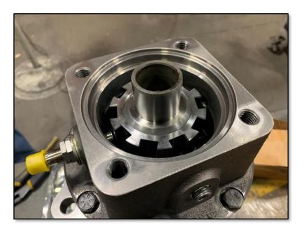
Once the Sungear Adapter is installed, place the small diameter O-Ring onto the Hydraulic Motor as shown in the photo below.
