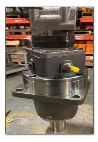
Verify that the orientation of the Hydraulic Motor, Motor Adapter, and Gearbox are all the same, as shown above.
