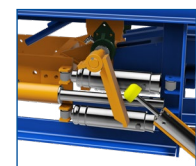
Air take-up for reliable performance and consistent tension for longer chain life.
