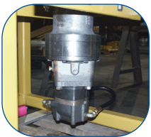
Heco direct drive gear box with hydraulic motor.
