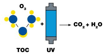
Sonny's Poseidon patented odor control system uses Ozone (O<sub>3</sub>) and UV Light to oxidize odor causing Total Organic Compounds (TOC) down to Carbon Dioxide (CO<sub>3</sub>) and Water (H<sub>2</sub>O).
