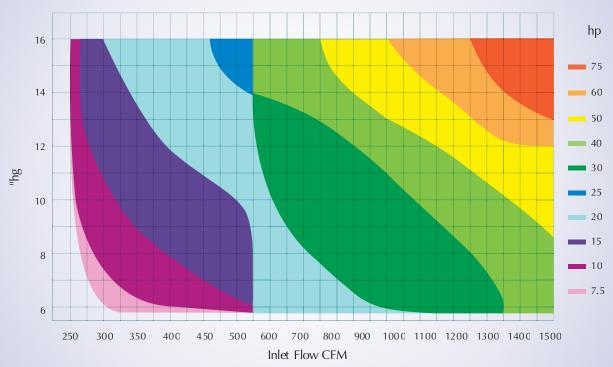
Performance based on inlet air at standard temperature of 68 ?F, an ambient pressure of 14.7 psia and 36% relative humidity. For performance at non-standard conditions, contact your authorized AVI representative.
