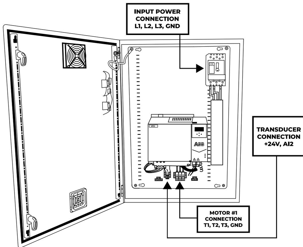
**To connect package to the power supply, motor and pressure transducer, please refer to picture below and Auto Cad drawings submitted in Chapter 4.**
