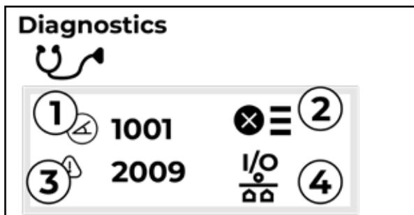
1. Active Fault - Shows the fault code
