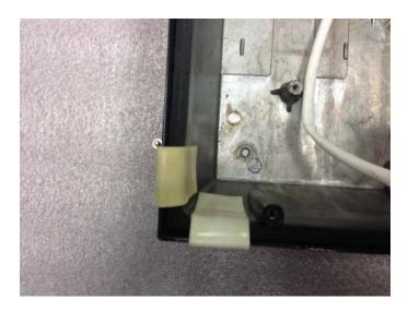
Place a small ring of silicon around each of the four fixture mount holes, on the mating surface of the housing boss.
