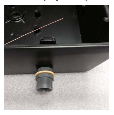
Insure fitting is tightened snug and properly compresses yellow washer.
