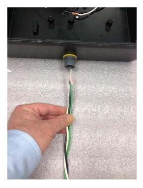
Slide grip claw, seal and cap nut onto cord.
