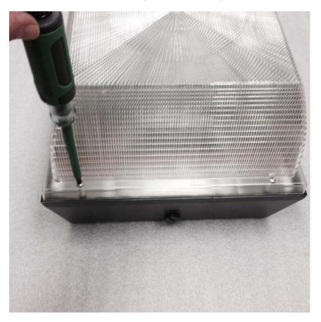
Screws are retained on lens cover with rubber washers.
