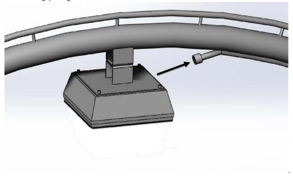
Feed cord through threaded fitting and conduit in the arch to junction box on opposite side of vertical stanchions.
