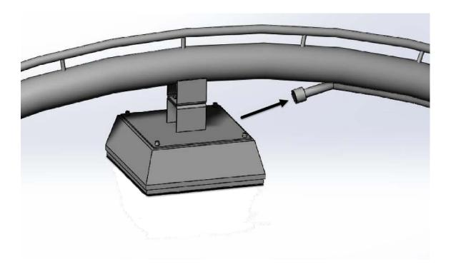
Tighten coupler into arch conduit and insure yellow washer is properly compressed.
