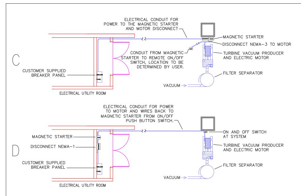
BASIC ELECTRICAL LAYOUTS WITH MAGNETIC STARTER
