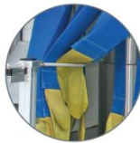
Optional Tire Shine retract lifts chamois above wheel well to allow online dressing application. Full retract also available for pickup truck beds.
