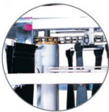
Adjustable wringing mechanism keeps each of the 24 overlapping synthetic chamois cloths ready to dry.
