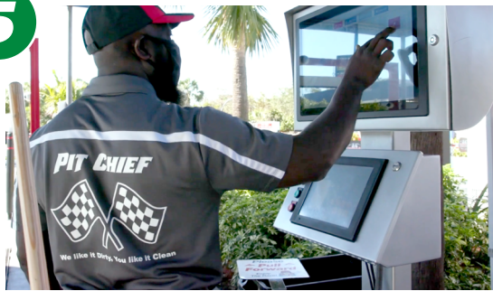
The easy drag-and-drop feature allows attendants to reorder queue, send rollers or start/stop the conveyor.
