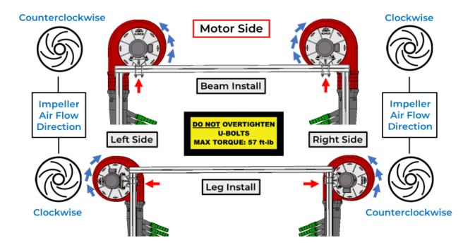
Only Use the Given Impeller Configurations to Insure Blower Optimization
