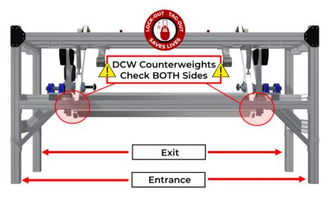
3. Using a ladder, get close to the Counterweight Assembly and look at where the Stainless Steel Angle attaches to the Aluminum H-Frame.
